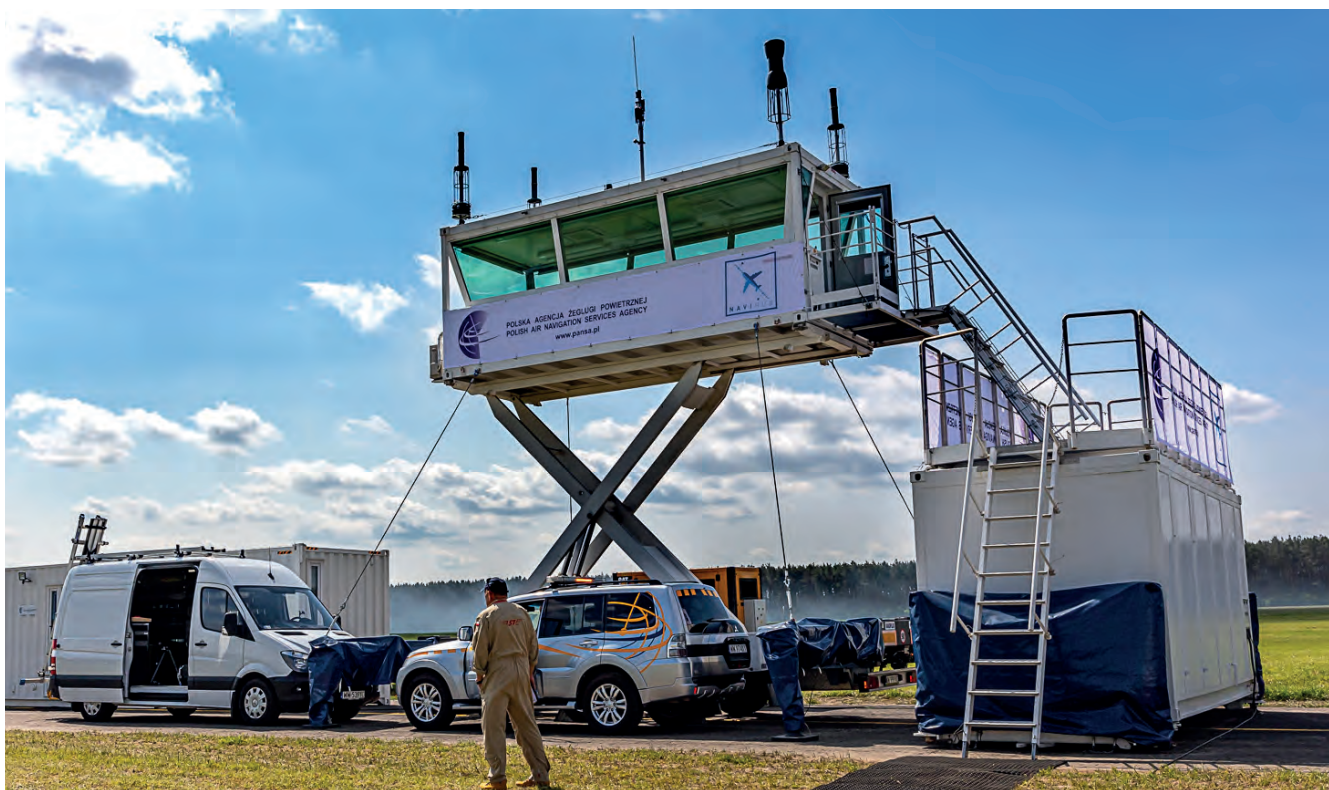
The PANSA mobile air traffic control tower at the airport in Kakolewo
