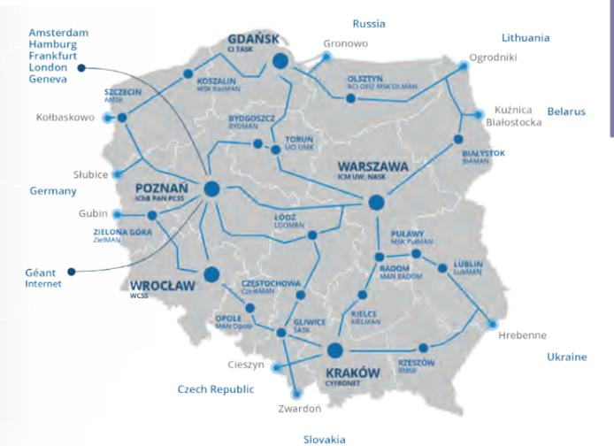
Fig. 3. PIONIER national optical backbone
